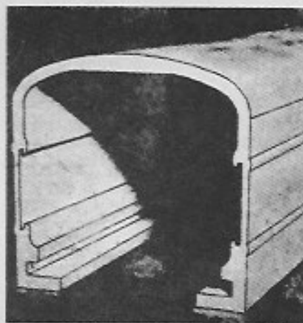
End view of extruded aluminum alloy coach body section showing window strip and floor support grooves. Patents pending.
