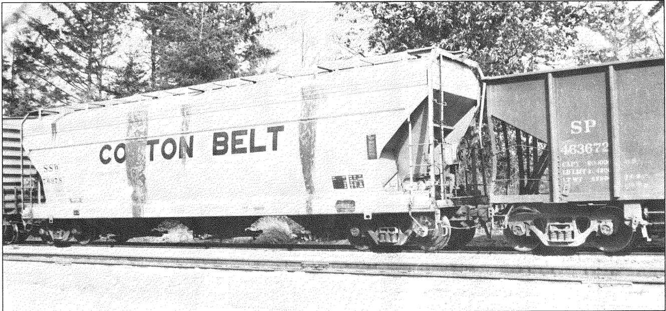
Cotton Belt #76978, built in 8/71, has newer horizontal ribs, but still has lower single rib. Photo at North Bend, Oregon —1989
