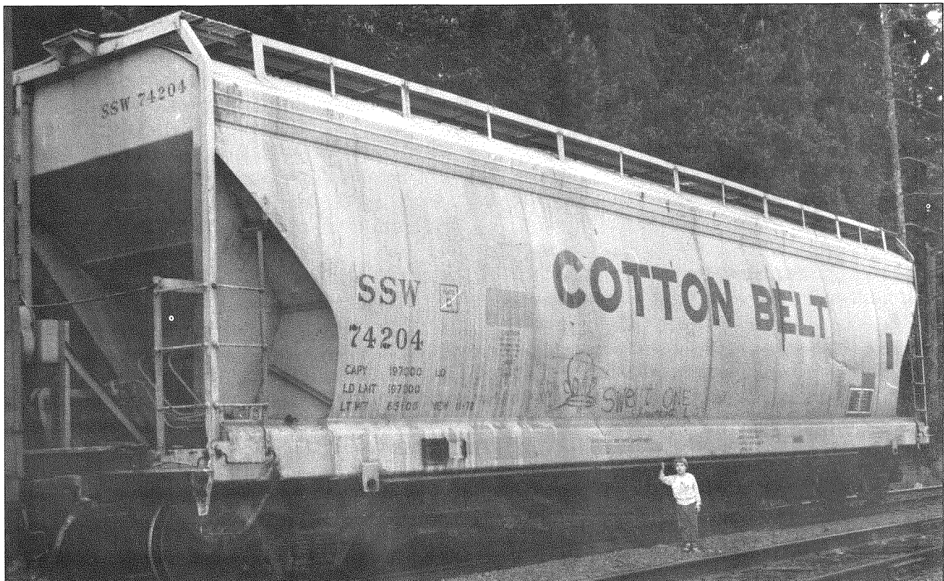
Cotton Belt # 74204, built in 11/72, with new rib section, lower rib not used. Photo at North Bend, Oregon —1989
