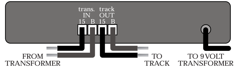
6-7 LocoMatic Controller wiring
