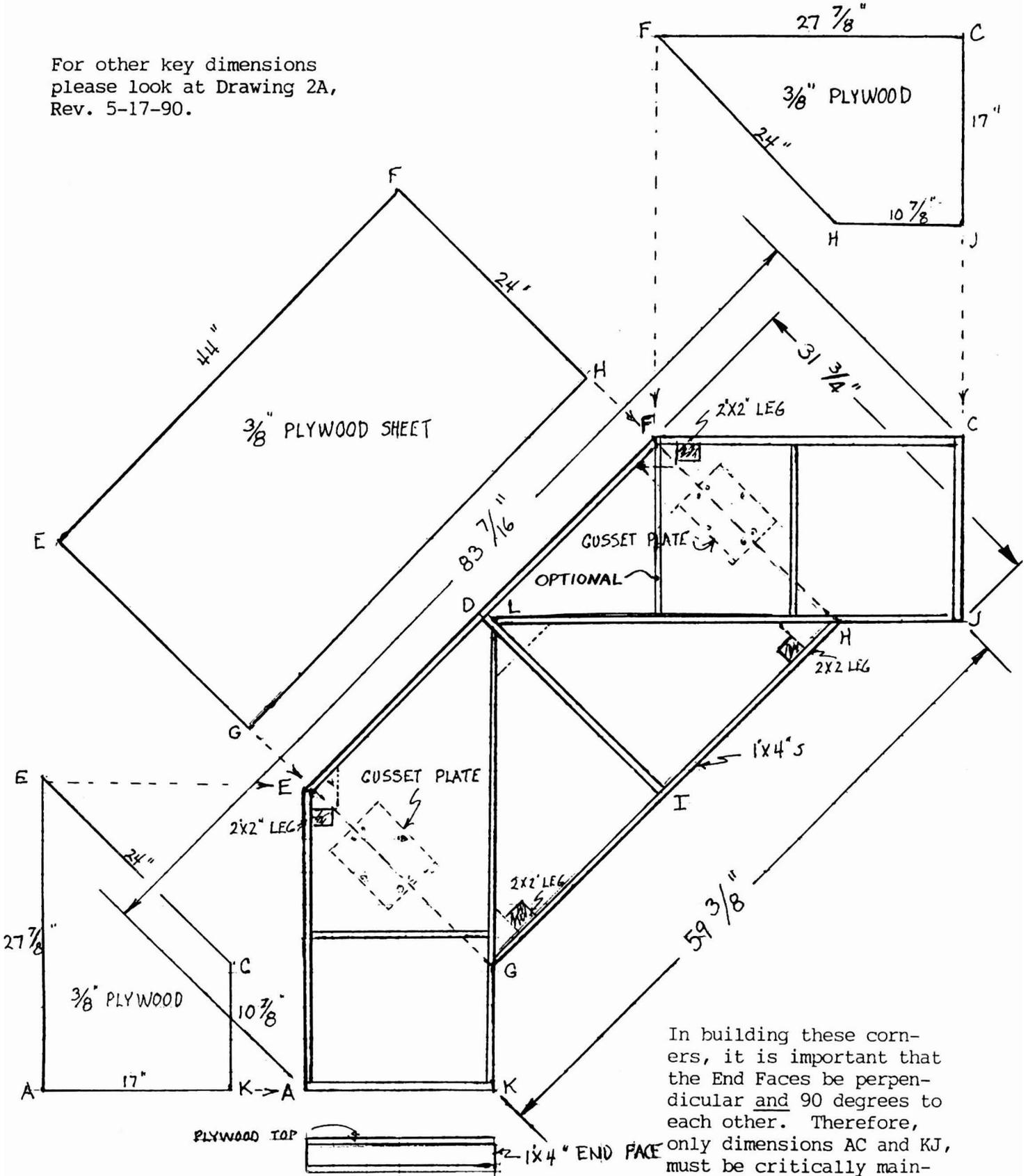
In building these corners, it is important that the End Faces be perpendicular and 90 degrees to each other. Therefore, only dimensions AC and KJ, must be critically maintained (top and bottom).
