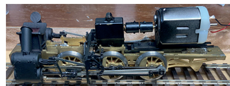
The prototype chassis for Simon Parent's run of CNR O-18 0-6-0s runs every bit as well as it looks.
