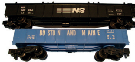
An American Models 50 foot rib-side boxcar above an AF 40 foot boxcar shows the size difference between contemporary and steam-era equipment.
