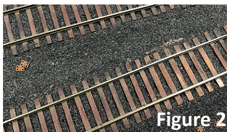
Figure 2 Little piles of tie plates identify the centers of hidden uncoupling magnets.
