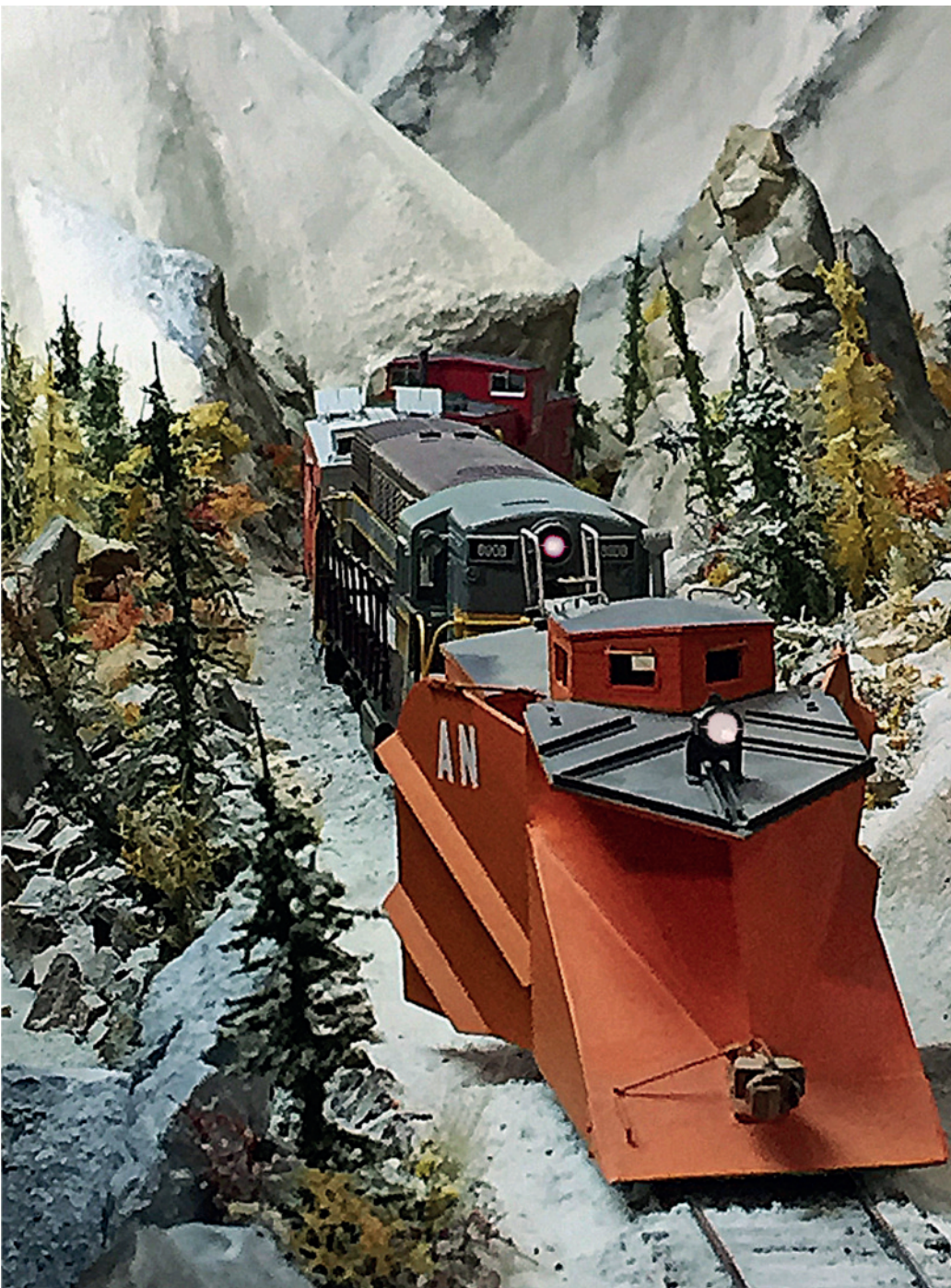
The railroad is in a constant battle with the elements on the Athabasca Northern. Snow drifts at Anaktuvuk Pass have brought out an open winged snow plow, the railroad's primary weapon in the fight. The snow plow was built from a Northeastern Scale Models kit and is based on a Boston and Maine Railroad prototype.
