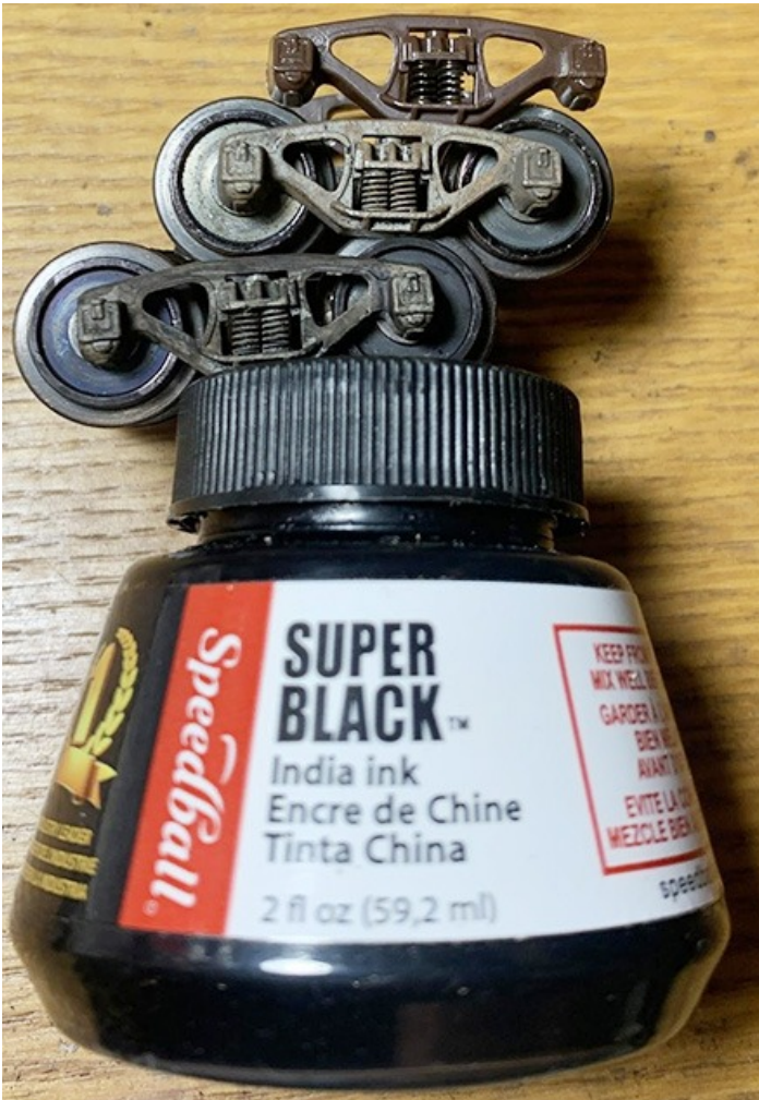
The photo above is a comparison of three trucks. First is the unpainted plastic, second is a painted truck with weathering ink, and the third has been treated with a wash of diluted India ink. I decided to further darken the trucks. Only a few minutes are needed to enhance truck details.
