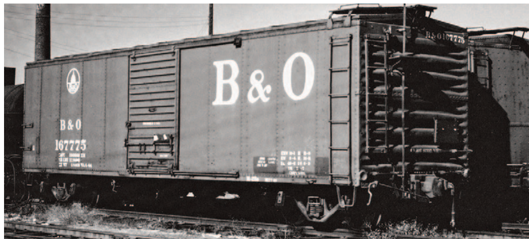
PHOTO 2 – The American Flyer box car shell closely approximates this B&O Class M-25 car. Notice the smooth sides, peaked roof and dreadnaught end panels. This example has a vertical brake wheel, but many were converted to horizontal wheels as these lasted into the early 1970s. Photo by Charles Mahan, Jr, from the author’s collection.
