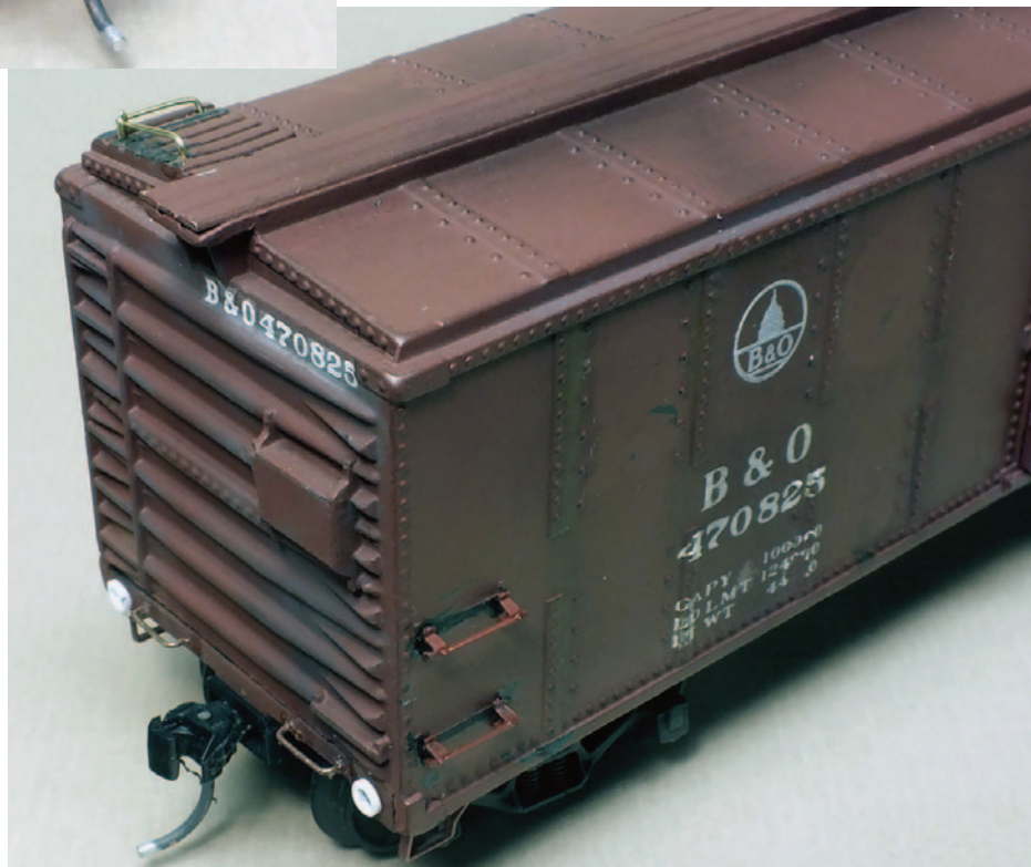
PHOTO 5 - Two grabs from PRS replaced the cast-on grabs which were carefully shaved off the car sides using a chisel blade. The PRS corner steps are just visible in this view.
