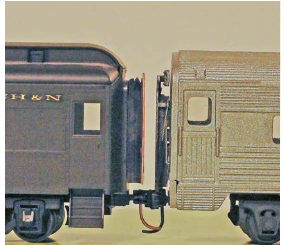
Coupled cars: Kadee 802 on left-hand car, Evolution on right.
