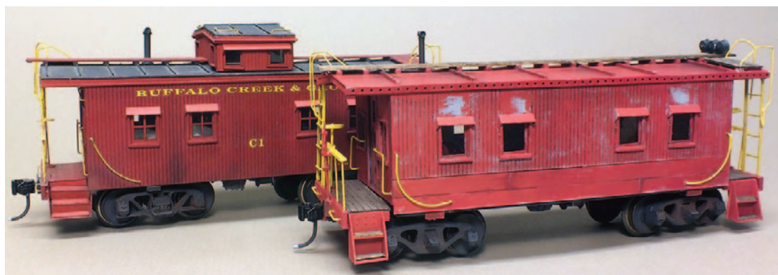
5. The differences between the I-1 "wide platform" (background) and I-5d "narrow platform" (foreground) are apparent in this photo. Notice that on the model, like the prototype, it was necessary to narrow the corner steps to accommodate the relocated trucks. On the I-5d the fasteners along the roof eave are Archer Fine Transfers rivet decals applied over the red paint.
