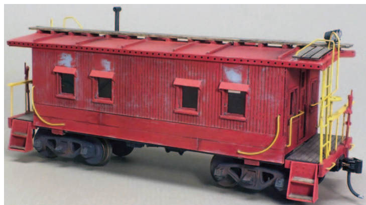
4. The model was brush painted with Vallejo Flat Red over grey primer. The handrails were fabricated from .020" wire painted Model Masters yellow. The red brake release valve and whistle on the end railing were scratch built as were the unique lights on the roof. American Models caboose trucks and Kadee 802 couplers complete the model.
