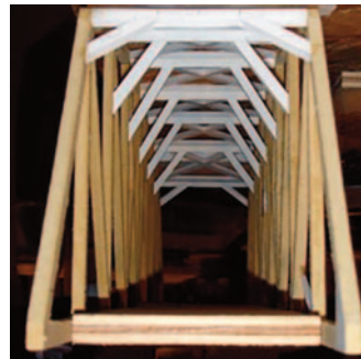
K-traces glued in place
