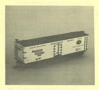
Many detail parts, such as door hardware, ladders, and steps are Grandt-Line castings of exquisite quality and detail. Air hoses were of Tomalco manufacture as were various pipe fittings supplied for underbody detail. Grab irons were extremely fine and pre-formed wire.
